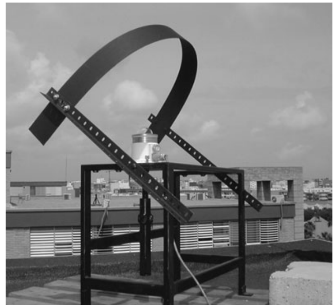
Figure 1. Experimental arrangement used to measure diffuse UVER.
